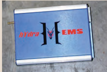
The engine is controlled by a Hydra Nemesis ECU from Flyin' Miata. This gives full control over every aspect of the motor and unlocks a lot of power.
