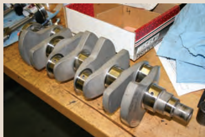
The Flyin' Miata stroker crankshaft started life as a 350 lb billet of steel. It helps increase displacement to 2020cc.
