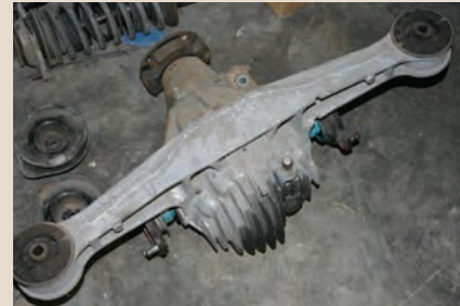
The car was built with an open differential originally, but a Torsen unit from a 2000 Miata was eventually installed.
