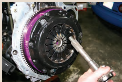
A 9.5 lb flywheel and a prototype clutch from Flyin' Miata take care of the power transfer.
