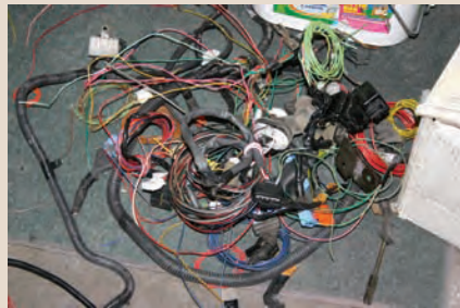
20-odd pounds of wire was removed from the car. A long job, it also simplified future troubleshooting.
