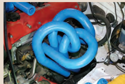
The header had to fit over 10' of fat tubing in the engine bay, making it a challenging job to squeeze in.
