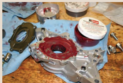
The oil pump was packed with assembly lubricant to ensure lots of oil pressure on startup.
