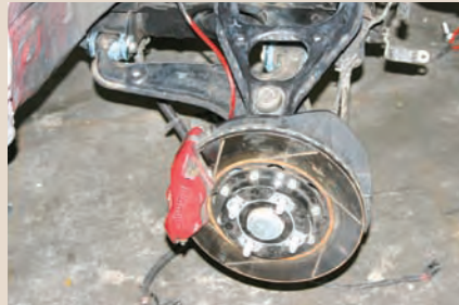
The brakes are a big brake kit from Flyin' Miata. They're lighter than the factory parts and the pads can easily be changed.
