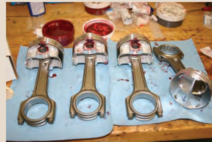
The pistons in the Flyin' Miata stroker kit are fairly exotic, very light with a short compression height.
