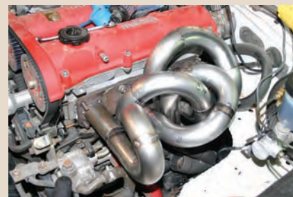
After the pipes were cut, the long process of TIG welding the header together began.
