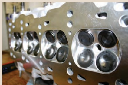
The head was ported and polished before being fitted with oversize valves and stiffer valve springs.
