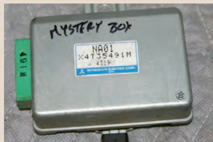
It's always important to label everything in a project like this! This turned out to be a cruise control brain.
