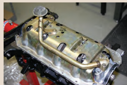
The Main Bearing Support Plate from a 2001 Miata was installed on the bottom of the engine.
