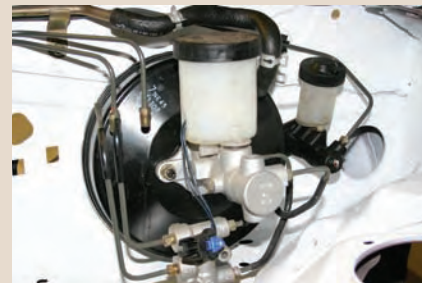
The 2005 master cylinder didn't quite line up with the 1994 brake lines. This is the sort of challenge involved in making a Frankenstein.
