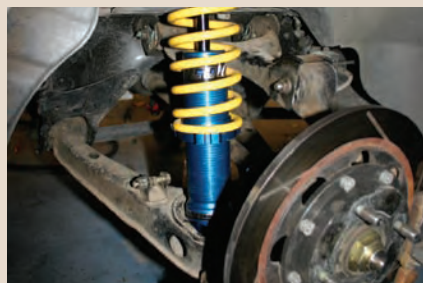
The springs and shocks underwent a lot of street and track testing before the final specification was decided.
