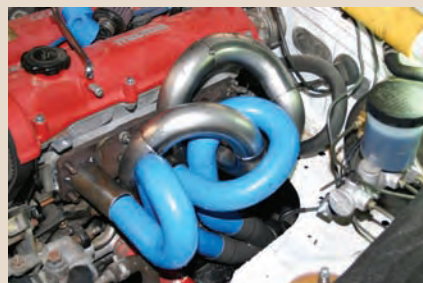
Halfway through building the header. The steel pipes are a good copy of the plastic.
