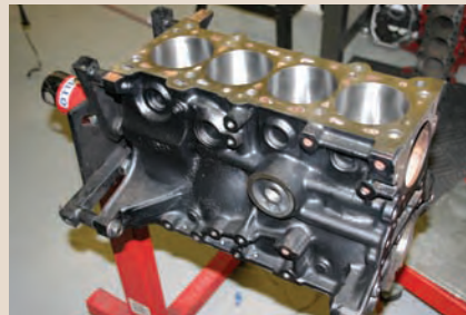
A carefully cleaned and bored engine block, ready for the build.
